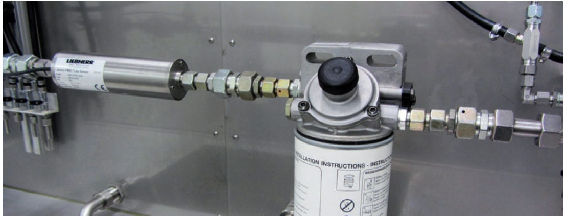
Litronic®-FMS III / RMH12 sensor integrated in a test and laboratory plant to monitor the demulsification capacity of a diesel fuel filter.
