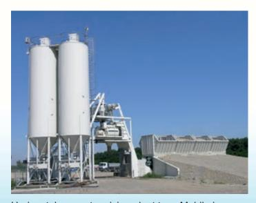
Horizontal concrete mixing plant type Mobilmix
