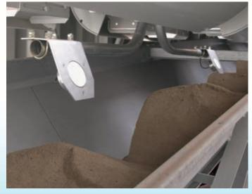
Moisture measurement of sand in a concrete mixing plant
